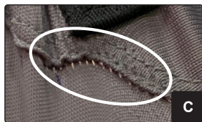
Seam slippage under load (Carer Side)
